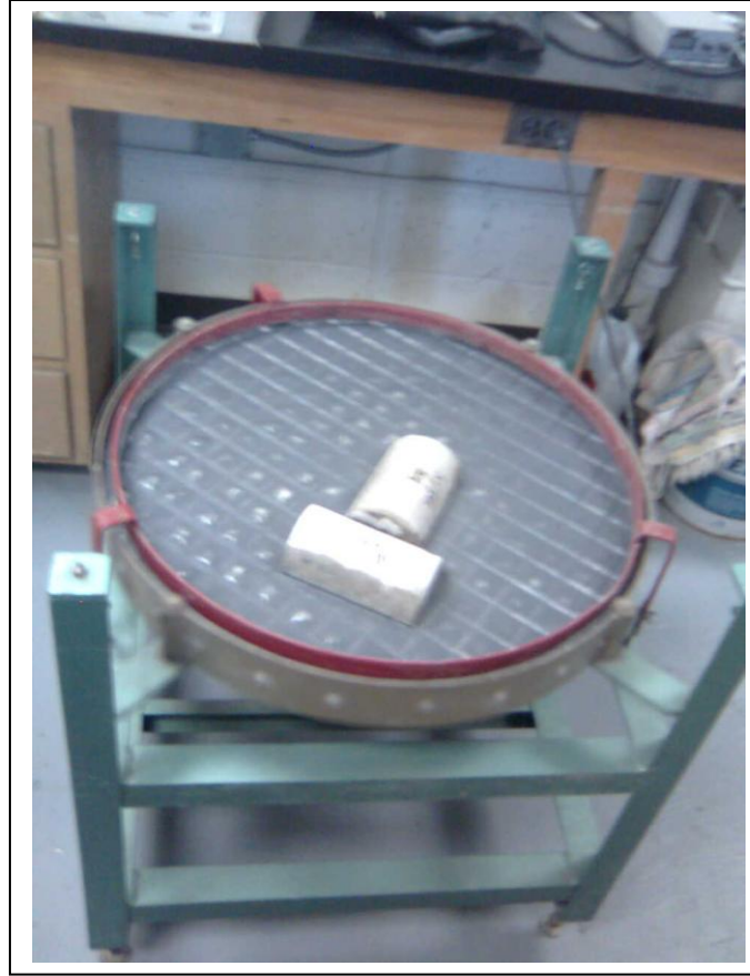
FIGURE 7 – Vibratory Table with Abrasives and Water as Lubricant
